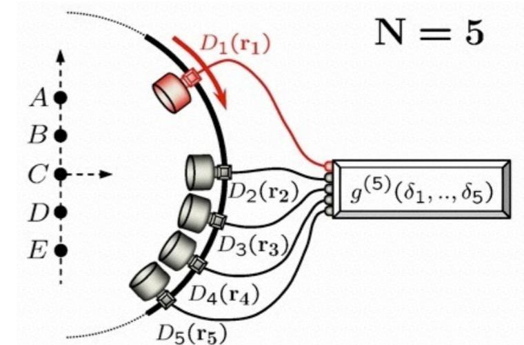
The modulation scales with  $N - 1$ , where  $N$  is the number of detectors. This allows us to measure the distance  $d$  between the sources with increased precision.
